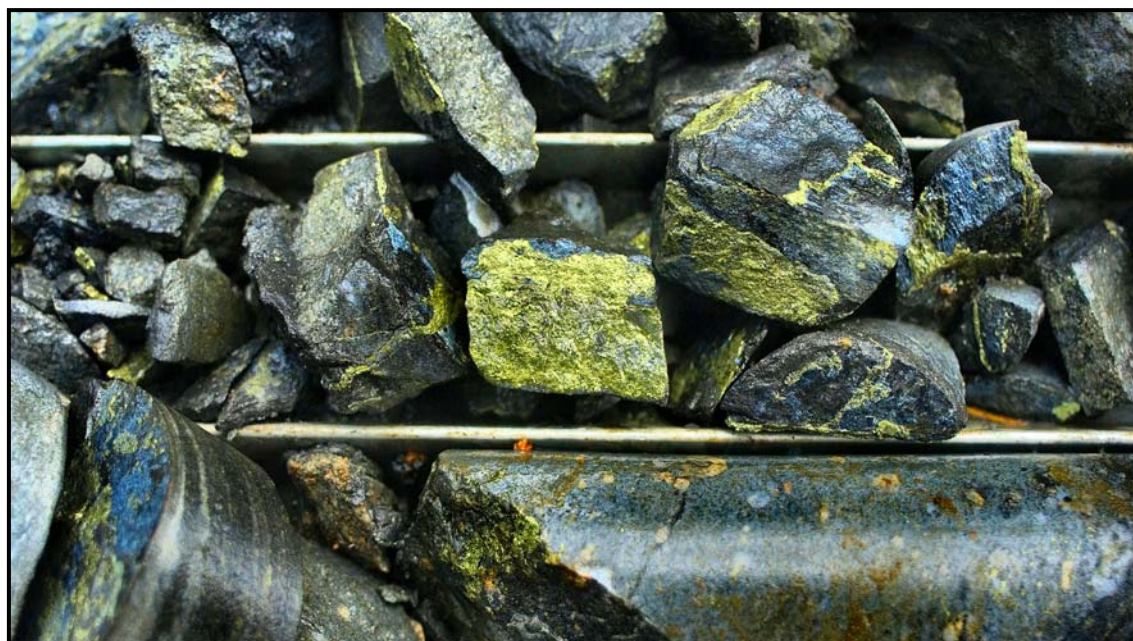
Figure 2: Core from Hole 07KTDH010 showing chalcopyrite mineralisation
