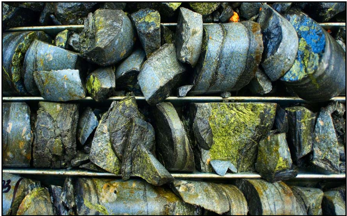
Figure 1: Core from Hole 07KTDH010 showing chalcopyrite mineralisation
